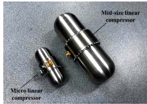
Fig. 19. A photograph of the developed micro linear compressor and the mid-size linear compressor.
